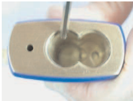
11 push down body and lock the shackle (still keep pushing down the shackle from this stage 11 to 14 stage)
