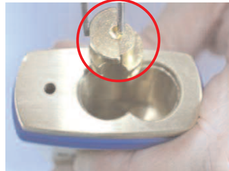
12 check the 2 locking balls and position
