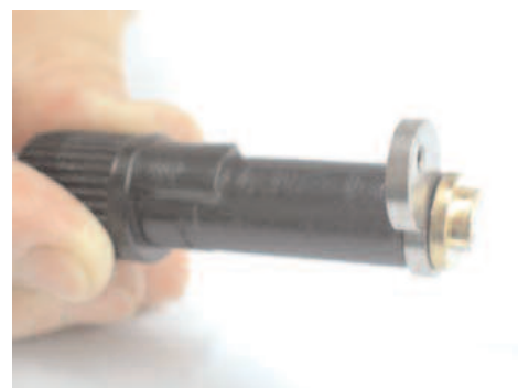
14 put the retained cam into cam hole according to the correct direction
