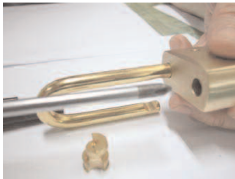
1 prepare tool and retained cam
