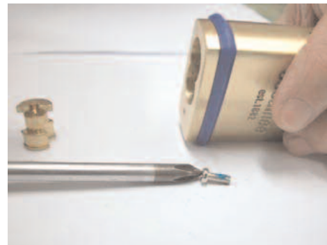
2 clockwise turn the tool to release shackle
