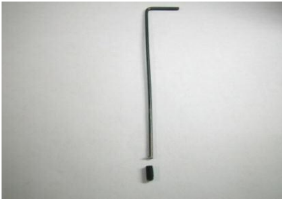
prepare Allen key and grub screw
