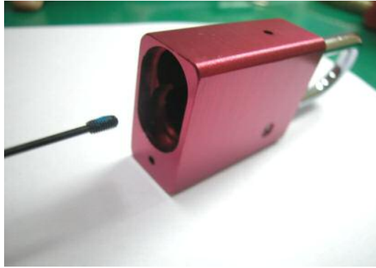
fix the grub screw on the screw hole of the cam to become key retained
