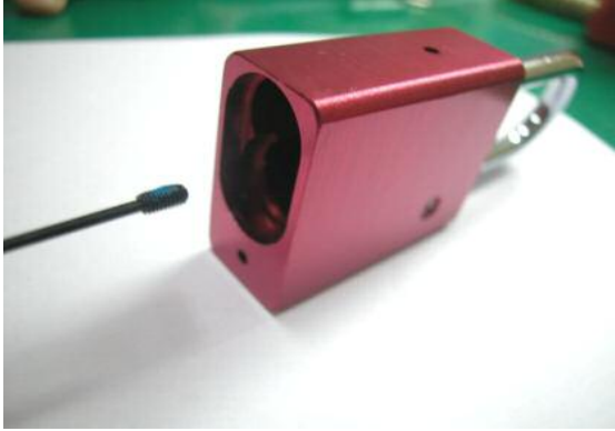
fix the grub screw on the screw hole of the cam to become key retained
