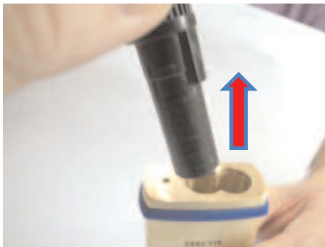
27 press down tightly then anti-clockwise turn the adjusting tool
